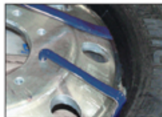
• Curved end For mounting and demounting top bead
